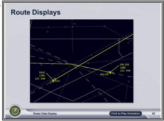
The route display program displays the route of a flight on the radar display, beginning with the position of the aircraft specified in the route display keyboard entry, and ending with the point on the route segment, which consists of keyboard-entered minutes, or a facility parameter amount of time in the future.
